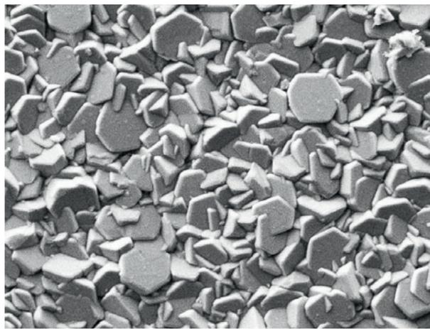
Figure 2:  $Al_2O_3$ -coating layer surface applied with MT-CVD
