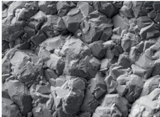
Figure 1:  $Al_2O_3$ -coating layer surface applied with HT-CVD
